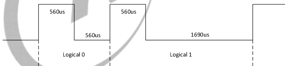
Figure 8-4 Logical '0' and Logical '1' of NEC Protocol
