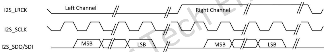
Standard I2S Timing Diagram
